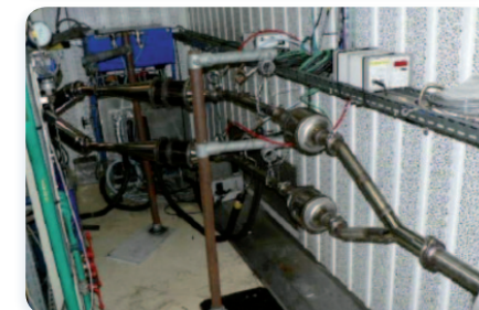
Engine Bench Test equipped with the ageing exhaust line (IJLRA, Renault)
